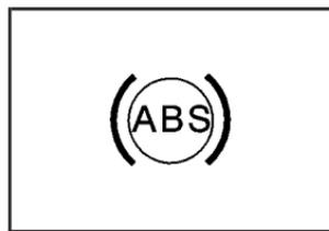
If there is a problem with the anti-lock brake system, this warning light will stay on. See *Anti-Lock Brake System Warning Light* on page 3-46.
