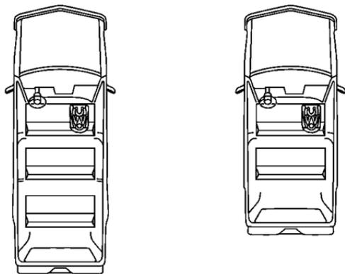
Your vehicle has a right front passenger air bag. A rear seat is a safer place to secure a forward-facing child restraint. See *Where to Put the Restraint on page 1-54*.
