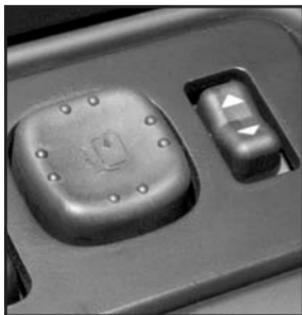
If your vehicle is equipped with power outside mirrors, the controls are located on the driver's door armrest.
