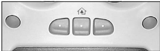
HomeLink<sup>®</sup> a combined universal transmitter and receiver, provides a way to replace up to three hand-held transmitters used to activate devices such as gate operators, garage door openers, entry door locks, security systems and home lighting. Additional HomeLink<sup>®</sup> information can be found on the internet at [www.homelink.com](http://www.homelink.com) or by calling 1-800-355-3515.
