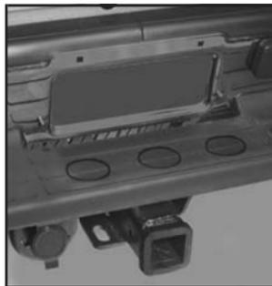
If you will be using the bumper to tow a trailer, and your step-bumper has three cutout circles you must push out the center cutout circle to install the trailer ball.
