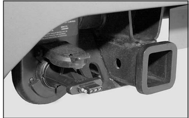
Connect the adapter with the tab pointing up (see arrow). The flip cap on the vehicle's seven-wire harness will lock onto the tab and help hold the adapter in place. Plug the four-way round pin connector onto the adapter.
