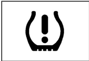
When the tire pressure monitoring system warning light is lit, one or more of your tires is significantly under-inflated.
