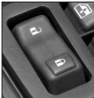
If your vehicle is equipped with power door locks, press the raised side of the switch, with the lock symbol, on either front door to lock all the doors at once.
