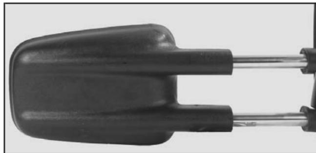
If your vehicle is equipped with camper-type mirrors, they can be adjusted so you can have a clear view of the objects behind you.
