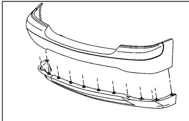
The front bumper lower air dam is held in place by a series of push-pins located around the lower edge of the front bumper. The push-pins are accessible from underneath the front bumper.
