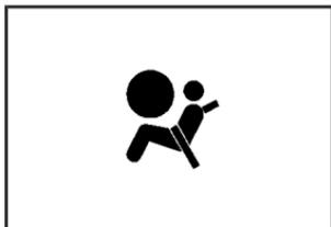
This light will come on when you start your vehicle, and it will flash for a few seconds. Then the light should go out. This means the system is ready.
