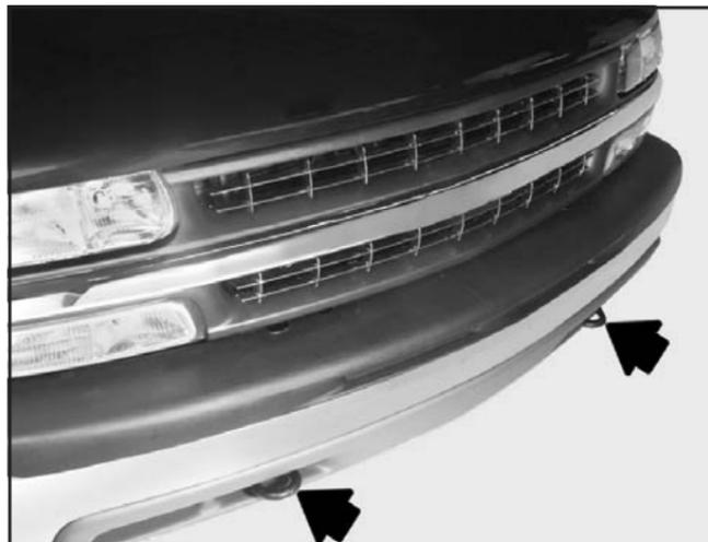
Your vehicle may be equipped with recovery hooks. The hooks are provided at the front of your vehicle. You may need to use them if you are stuck off-road and need to be pulled to some place where you can continue driving.
