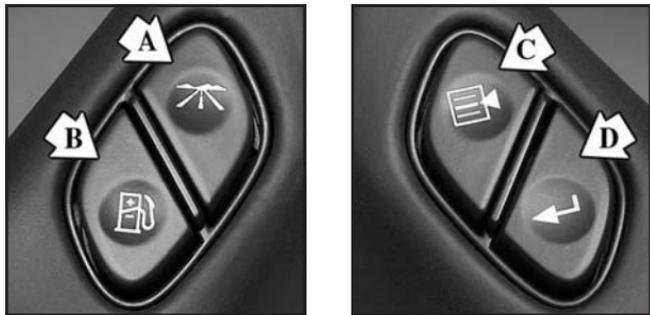
**A (Trip Information):** This button will display the odometer, personal trip odometer, business trip odometer, hourmeter, annual log and the timer.
