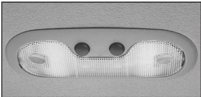
Your vehicle may also have reading lamps in other locations. To turn the lamps on or off, press the button located next to the lamp. The lamps are fixed and cannot be adjusted.
