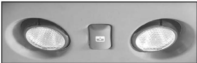
Your vehicle may be equipped with a power sliding sunroof. To open or close your sunroof, the ignition or RAP needs to be active. See “Retained Accessory Power” (RAP), under Starting and Operating Your Vehicle.
