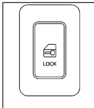
If your vehicle has this power door lock switch, press the bottom of the switch on either front door to lock all the doors at once.
