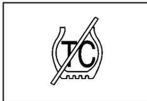
When the traction off light is on, the TAS is off and will not limit wheel spin. Adjust your driving accordingly.
