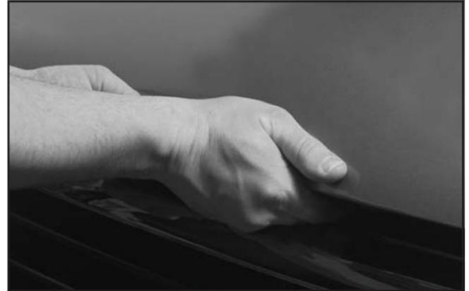
2. Then go to the front of the vehicle and pull up on the secondary hood release located near the center of the grill.
