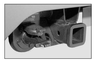
Connect the adapter with the tab pointing up (see arrow). The flip cap on the vehicle's seven-wire harness will lock onto the tab and help hold the adapter in place. Plug the four-way round pin connector onto the adapter.
