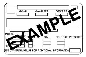
The Certification/Tire label is found on the rear edge of the driver's door or in the Incomplete Vehicle Document in the cab. The label shows the size of your original tires and the inflation pressures needed to obtain the gross weight capacity of your vehicle. This is called the GVWR (Gross Vehicle Weight Rating). The GVWR includes the weight of the vehicle, all occupants, fuel and cargo.
