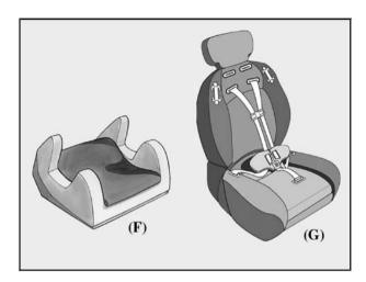
A booster seat (F-G) is a child restraint designed to improve the fit of the vehicle's safety belt system. Some booster seats have a shoulder belt positioner, and some high-back booster seats have a five-point harness. A booster seat can also help a child to see out the window.
