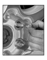
6. After mounting the spare, put the wheel nuts back on with the rounded end of the nuts toward the wheel. Tighten each wheel nut by hand. Then use the wheel wrench to tighten the nuts until the wheel is held against the hub.
