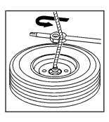
The wheel wrench has a hook that allows you to pull the hoist cable towards you to assist in reaching the spare tire.
