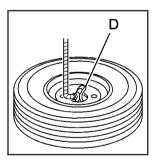
When the tire has been lowered, tilt the retainer (D) at the end of the cable so it can be pulled up through the wheel opening.
