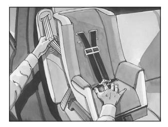
6. To tighten the belt, push down on the child restraint, pull the shoulder portion of the belt to tighten the lap portion of the belt and feed the shoulder belt back into the retractor. If you are using a forward-facing child restraint, you may find it helpful to use your knee to push down on the child restraint as you tighten the belt. You should not be able to pull more of the belt from the retractor once the lock has been set.
