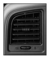
Use the air outlets located in the center and on the side of your instrument panel to direct the airflow.
