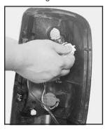
4. Pull the old bulb straight out from the socket.
