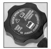
Then replace the pressure cap. Be sure the pressure cap is hand-tight and fully seated.
