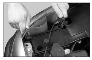
Your vehicle is equipped with two pins, remove the two pins on the top of the headlamp assembly.
