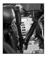
Connect the other end of the negative (–) cable to the remote negative (–) terminal, marked GND, on the vehicle with the dead battery.
