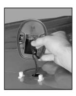
4. Put a new bulb into the socket and turn clockwise until it locks in place.
