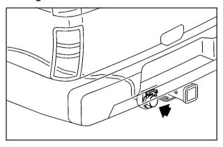
Your vehicle is equipped with the seven-wire trailer towing harness. This harness with a seven-pin universal trailer connector is attached to a bracket on the hitch platform.
