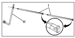
Attach the wheel wrench (H) and extensions (I) together.
