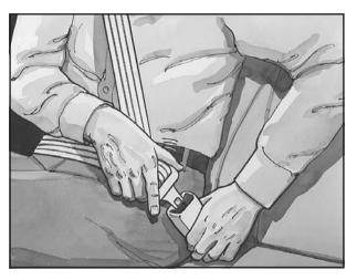
Pick up the latch plate and pull the belt across you. Do not let it get twisted. 2. Push the latch plate into the buckle until it clicks.
