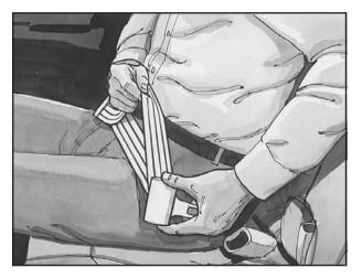
A lap safety belt does not have a retractor. To make the belt longer, tilt the latch plate and pull it along the belt.
