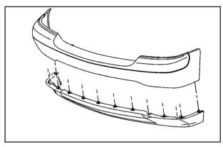
The front bumper lower air dam is held in place by a series of push-pins located around the lower edge of the front bumper. The push-pins are accessible from underneath the front bumper.
