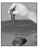
Remove the two screws and lift off the lens.
