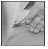
To fold, pull up on the strap loop at the rear of the seat cushion. Then, pull the seat cushion up and fold it forward.
