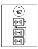
The transfer case buttons are located to the left of the instrument panel cluster.
