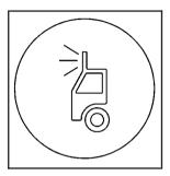
This switch is located on the center of the instrument panel near the comfort controls. When the switch wiring is connected to an auxiliary roof mounted lamp, pressing the switch will activate the lamp and illuminate an indicator light near the switch. Pressing the switch again will turn off the roof mounted lamp.
