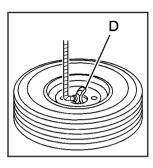
13. Tilt the retainer at the end of the cable and pull it through the wheel opening. Pull the tire out from under the vehicle.
