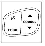
ردر : If your vehicle is equipped with the steering wheel control buttons you can use them to interact with the OnStar® system.
