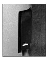
Pull the handle inside the vehicle located under and to the left of the steering wheel.
