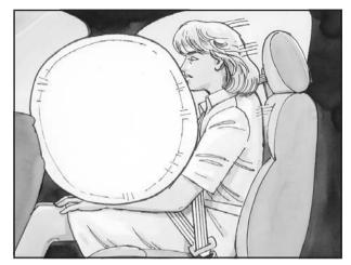
The right front passernger's frontal air bag is in the instrument panel on the passenger's side.
