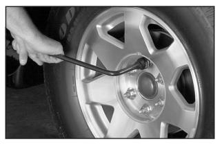
Use the wheel wrench to loosen all the wheel nuts. Turn the wheel wrench counterclockwise to loosen the wheel nuts. Don't remove the wheel nuts yet.
