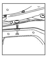
Pull the push-pins and lower air dam assembly away from the retainers until the lower air dam is free.
