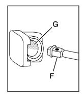
Insert the hoist end (F) through the hole (G) in the rear bumper and into the hoist shaft.
